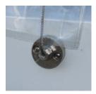
The Wire Ropes are of SS and the Guides are Nylon 66.
